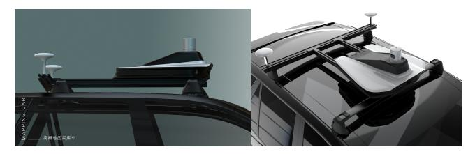
The mapping hardware kit leverages the early-fusion technology from passenger vehicle autonomous driving, and use Whale Dynamic's proprietary fusion box hardware to provide spatial-temporal synchronization, and fuse sensor data inputs from GNSS, Lidar, camera, and IMU sensors. Thanks to the accurate data fusion, high-quality raw dataset for HD map generation could be collected.
